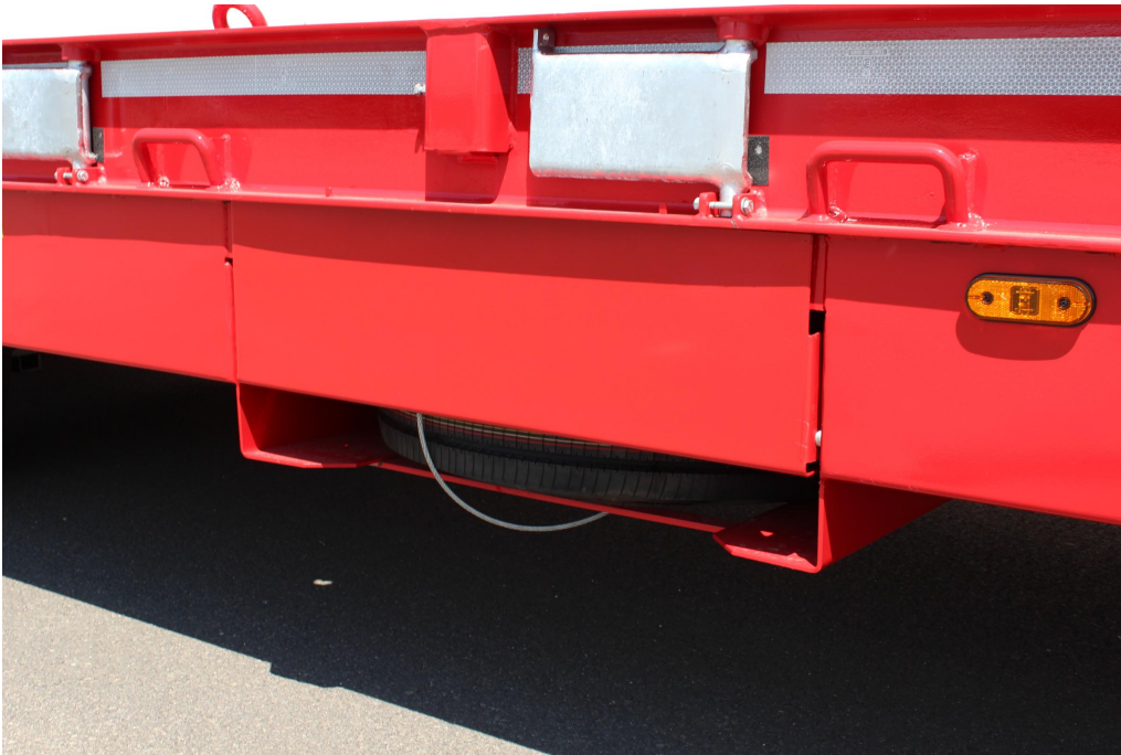
5 pairs of lashing points on the external frame
