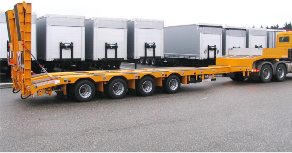
4-axle low loader semitrailer - reinforced - extendible
