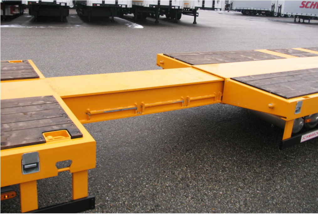
Pull-out central frame, incremental adjustment with pneumatic locking
