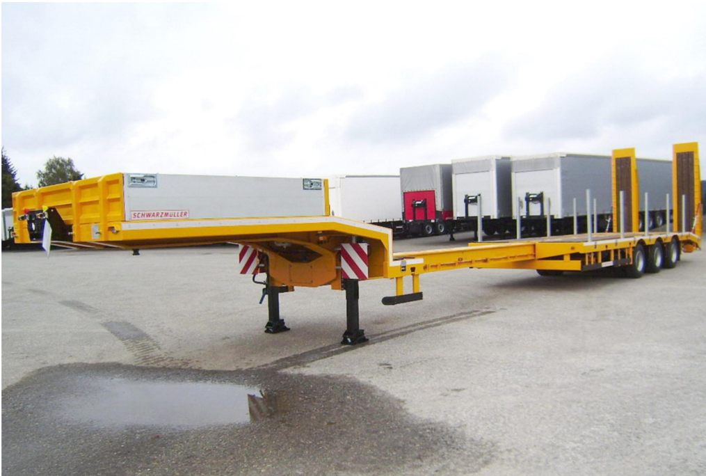
3-axle low loader semitrailer - reinforced - extendible
