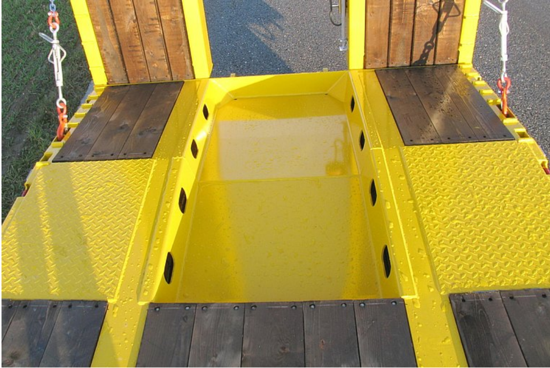
Excavator shovel recess between side members at rear
