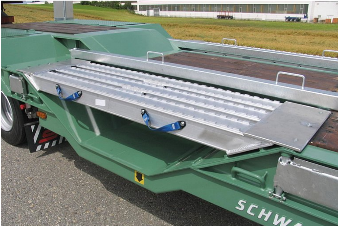
Wheel recesses integrated in external frame, coordinated with floor construction incl. drive-on aluminium cover
