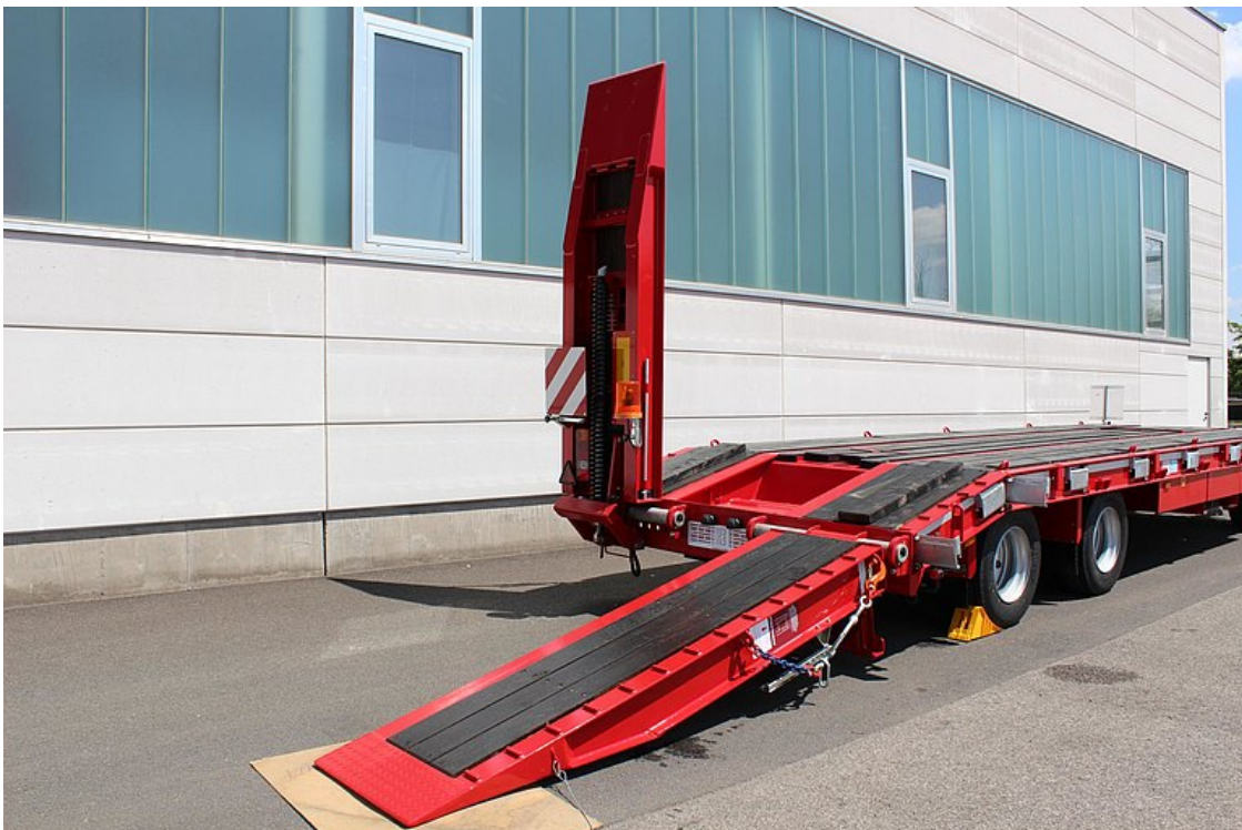
2 folding single-part loading ramps with hardwood flooring
