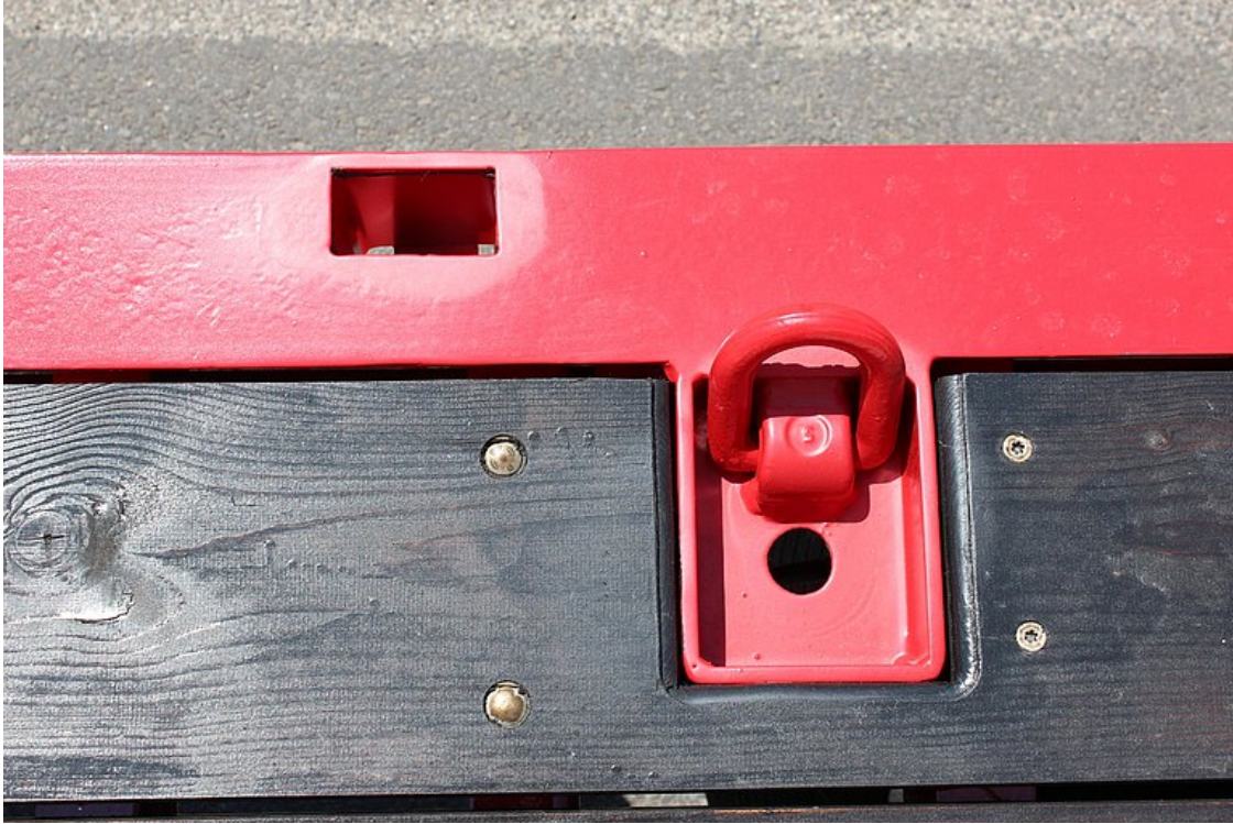
5 pairs of recessed, foldable lashing eyes
