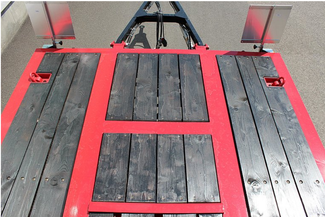
Waterproofed softwood floor, protruding beyond frame profiles
