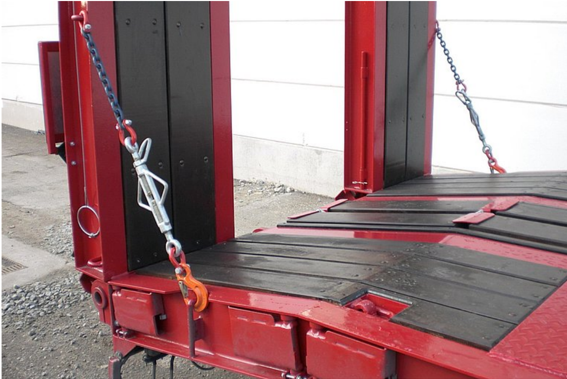
Additionally secured by the loading ramp chains for safe transport
