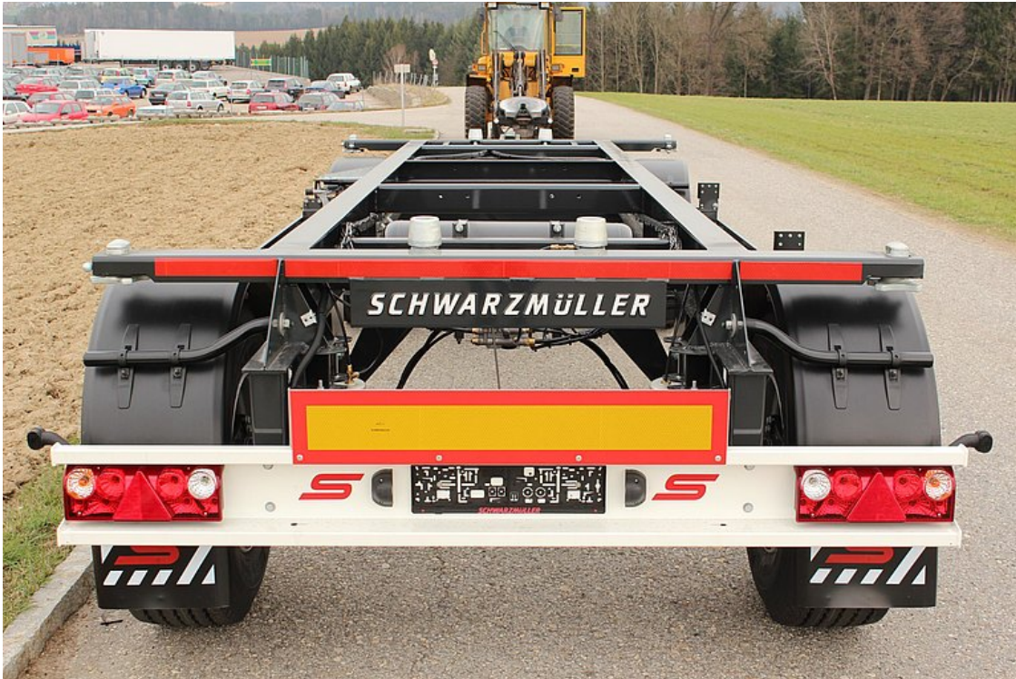
Underride protection incl. integrated light system
