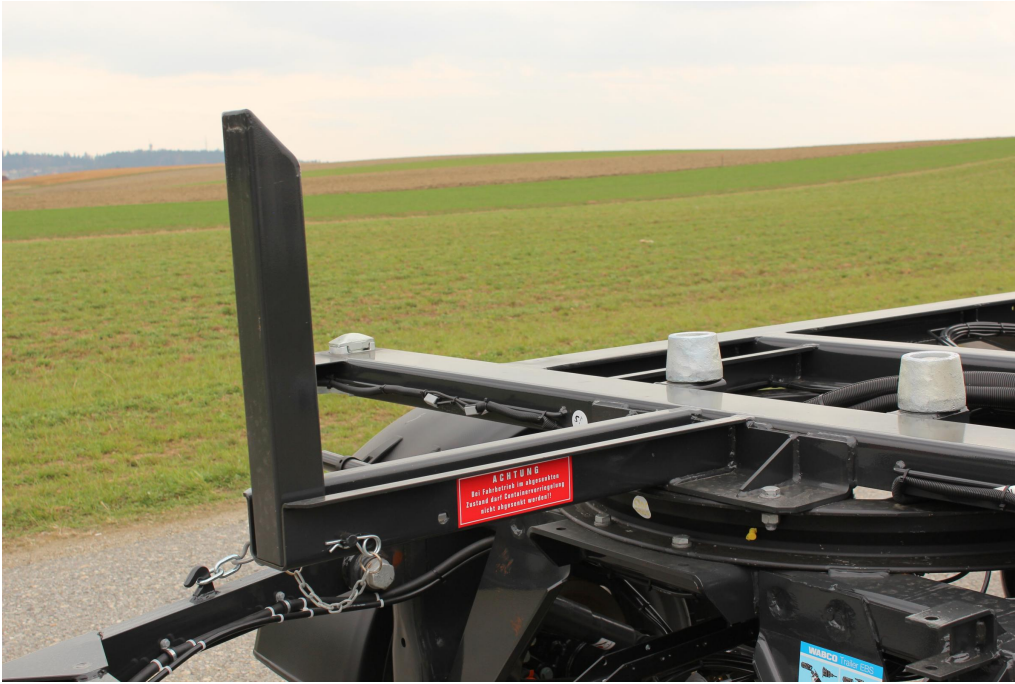
Stop support at front, tiltable and relocatable
