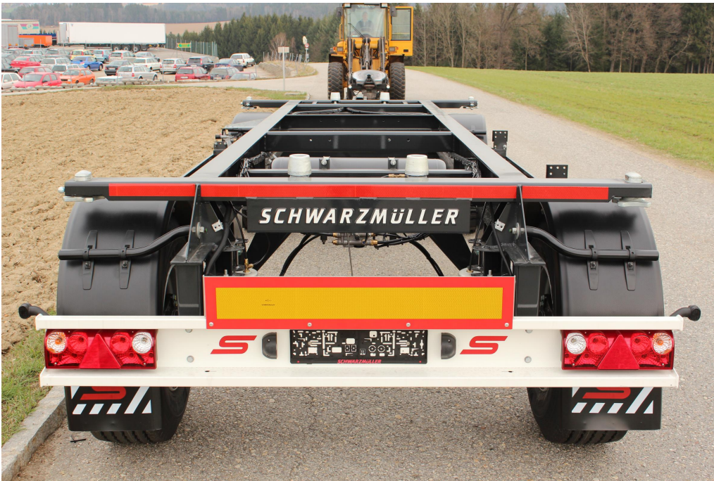
Underride protection incl. integrated light system
