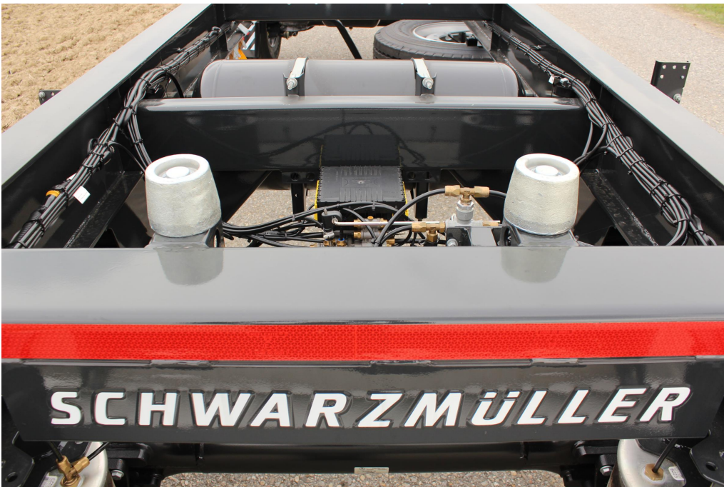
Support cross member incl. 4 container locks in accordance with EN 284 (20ft locking dimension)
