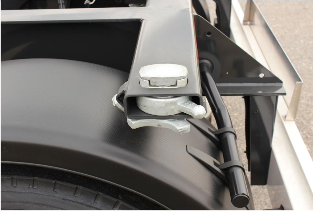
Support cross member incl. 4 container locks in accordance with EN 284 (20ft locking dimension)
