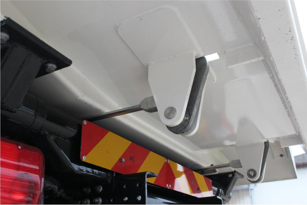
Automatic mechanical rear wall locking
