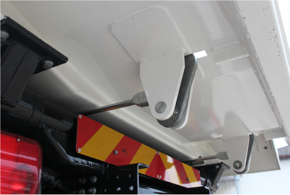
Automatic mechanical rear wall locking
