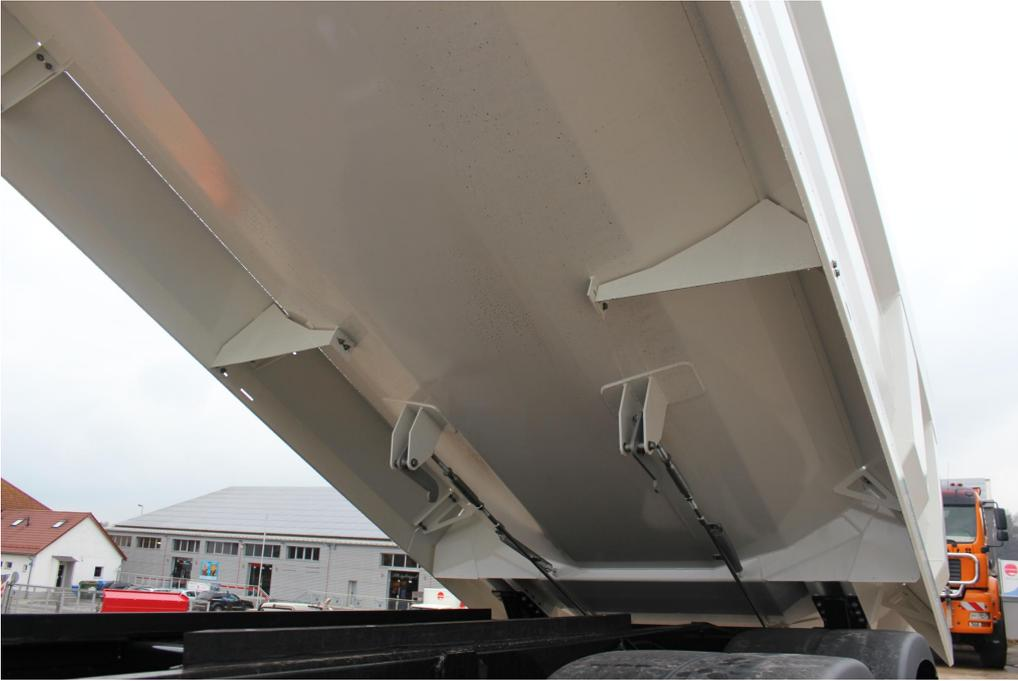
Specially canted body for maximum impact and wear protection
