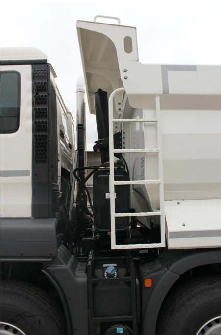
Specially canted Hardox body for maximum impact and wear protection
