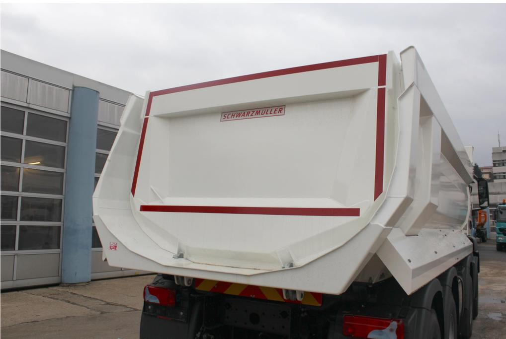
Steel plate rear wall = hinged wall with recessed bearing
