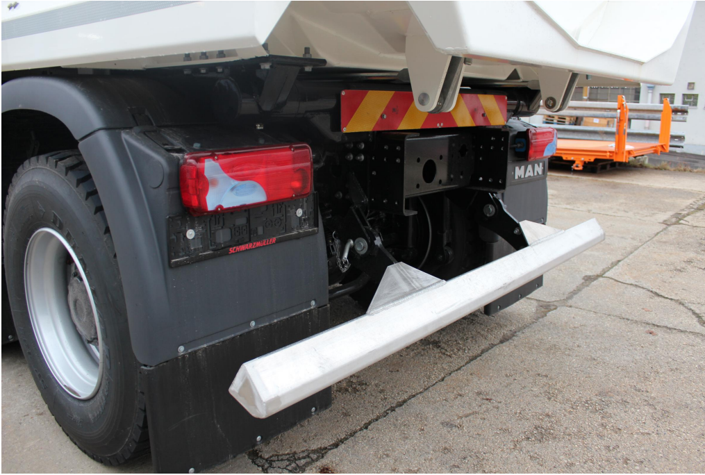
OPTIONAL: Foldable aluminium underride protection
