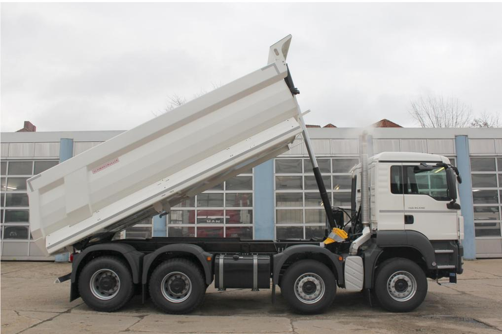
Steel segment tipper body on 4-axle truck
