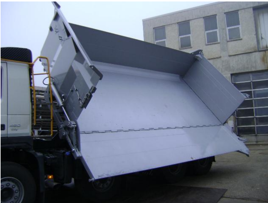
OPTIONAL: Foldable aluminium underride protection for road-finishing use
