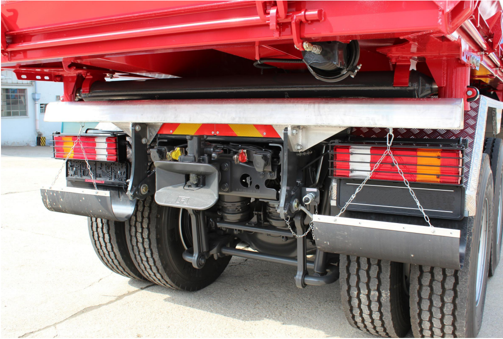
OPTIONAL: Foldable aluminium underride protection for road-finishing use
