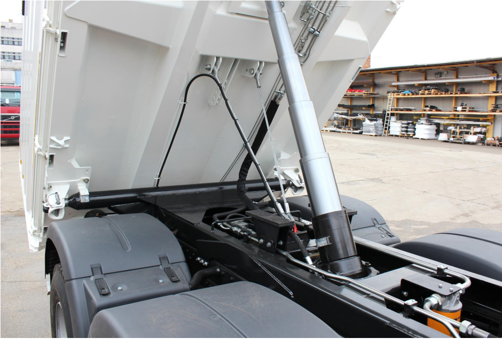
Hard chrome-plated, high-quality tilt cylinder
