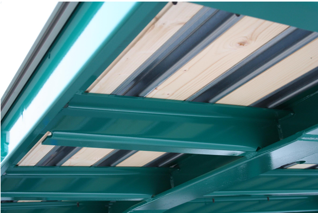
External frame with recessed 2.5 t lashing points
