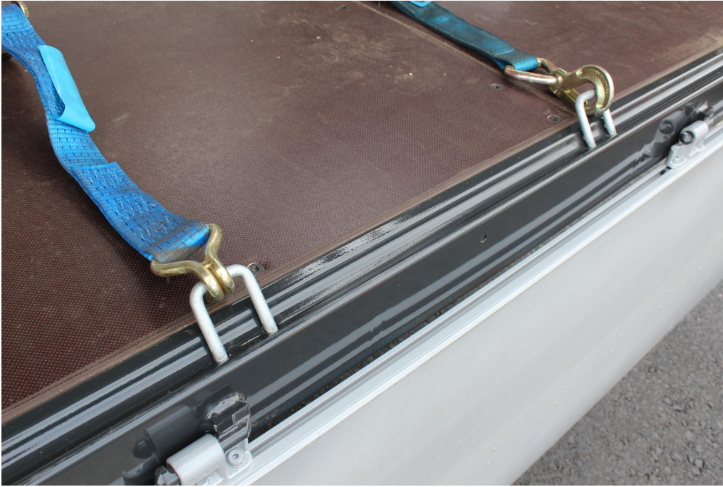
External frame with recessed 2.5 t lashing points
