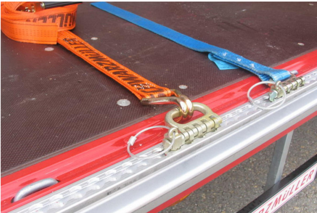
External frame with recessed 2.5 t lashing points
