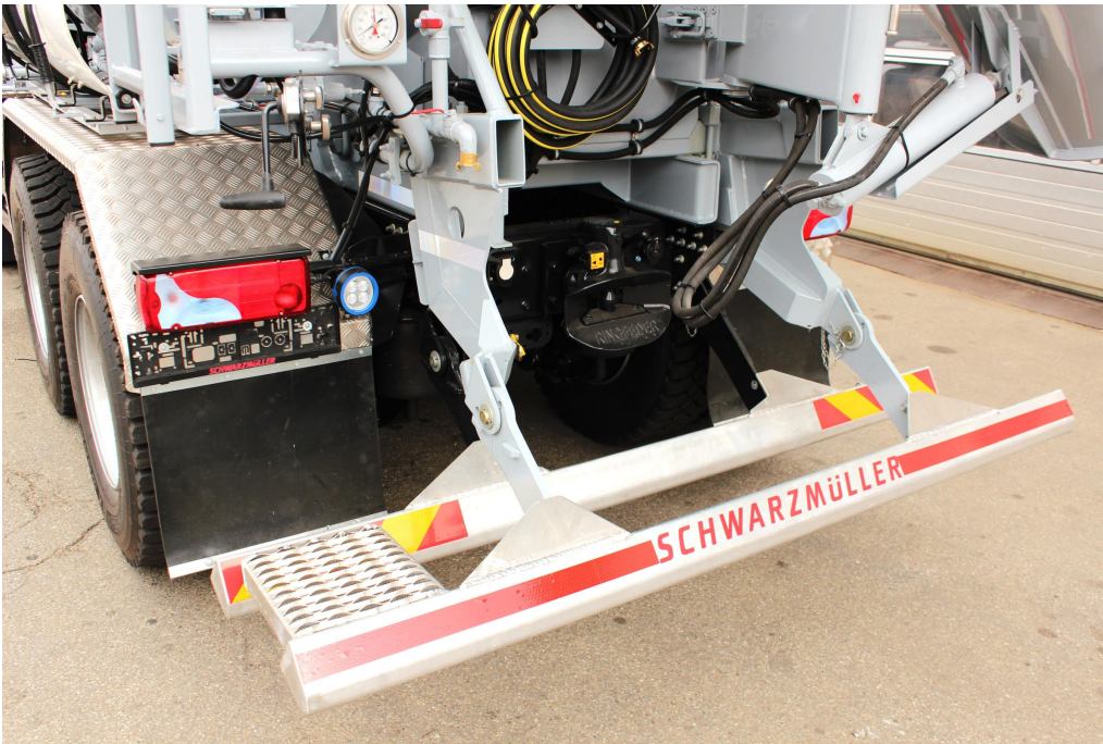
OPTIONAL: Foldable and removable underride protection
