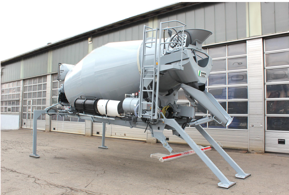
Rearward angled supports for secure body placement
