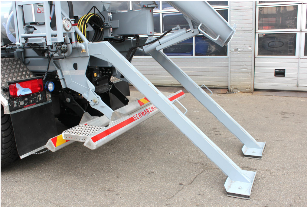
Rearward angled supports for secure body placement
