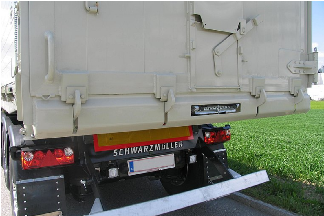
Combined rear wall incl. grain feeder and sliding step unit
