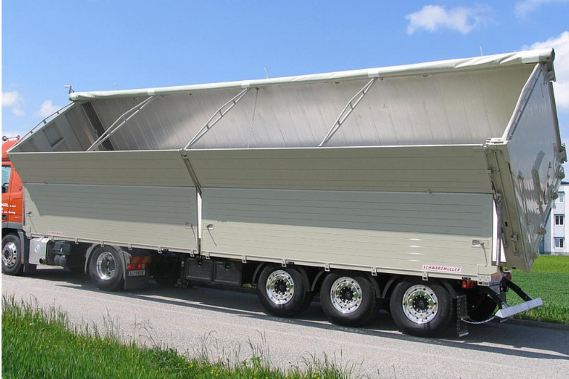
Can be used for various types of transport with (un)loading and tipping to the left or rear
