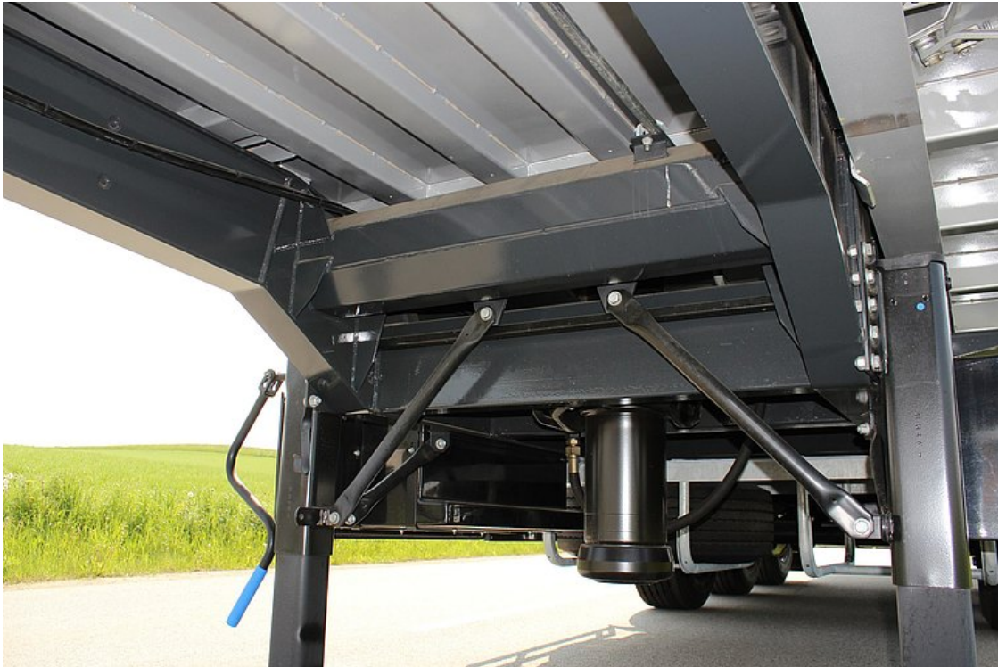
Stable and torsionally rigid chassis design with additional torsion tubes for 3-way tipping
