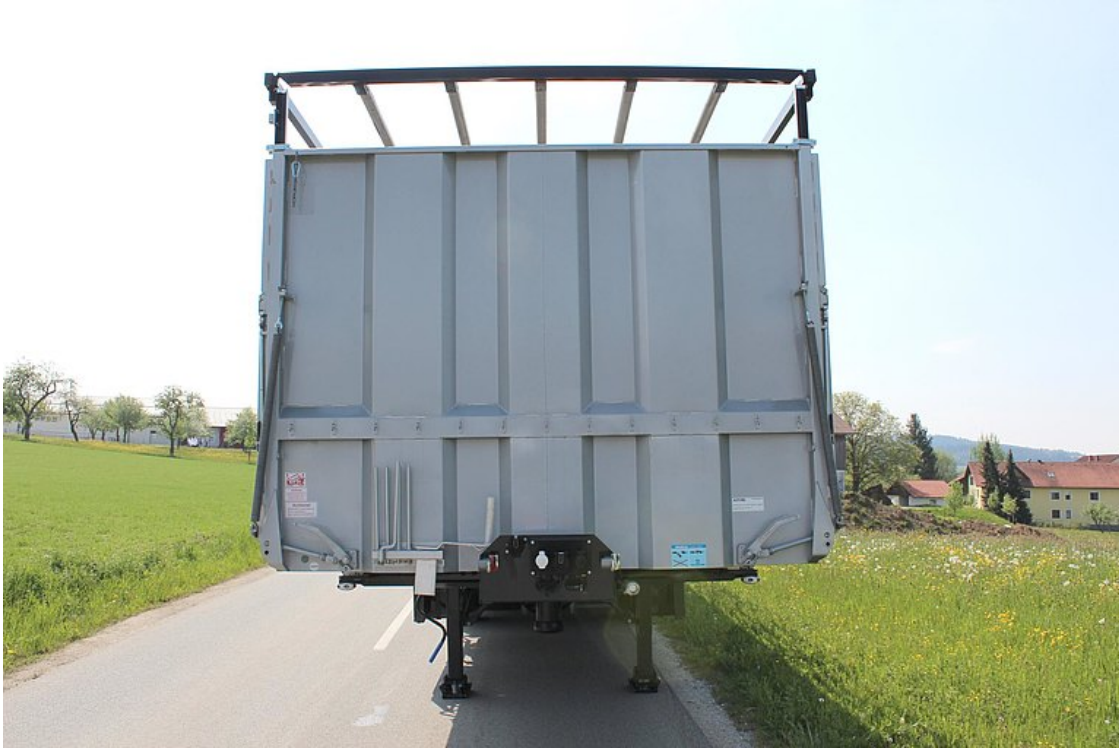
Fixed steel sheet front wall, 3 mm
