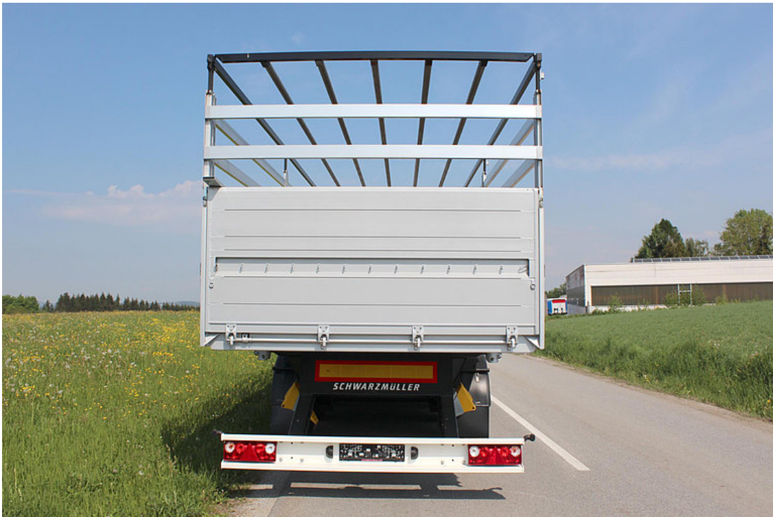
Aluminium hollow profile rear wall, folding with extended swivel bolt locks and hinged with man. central locking
