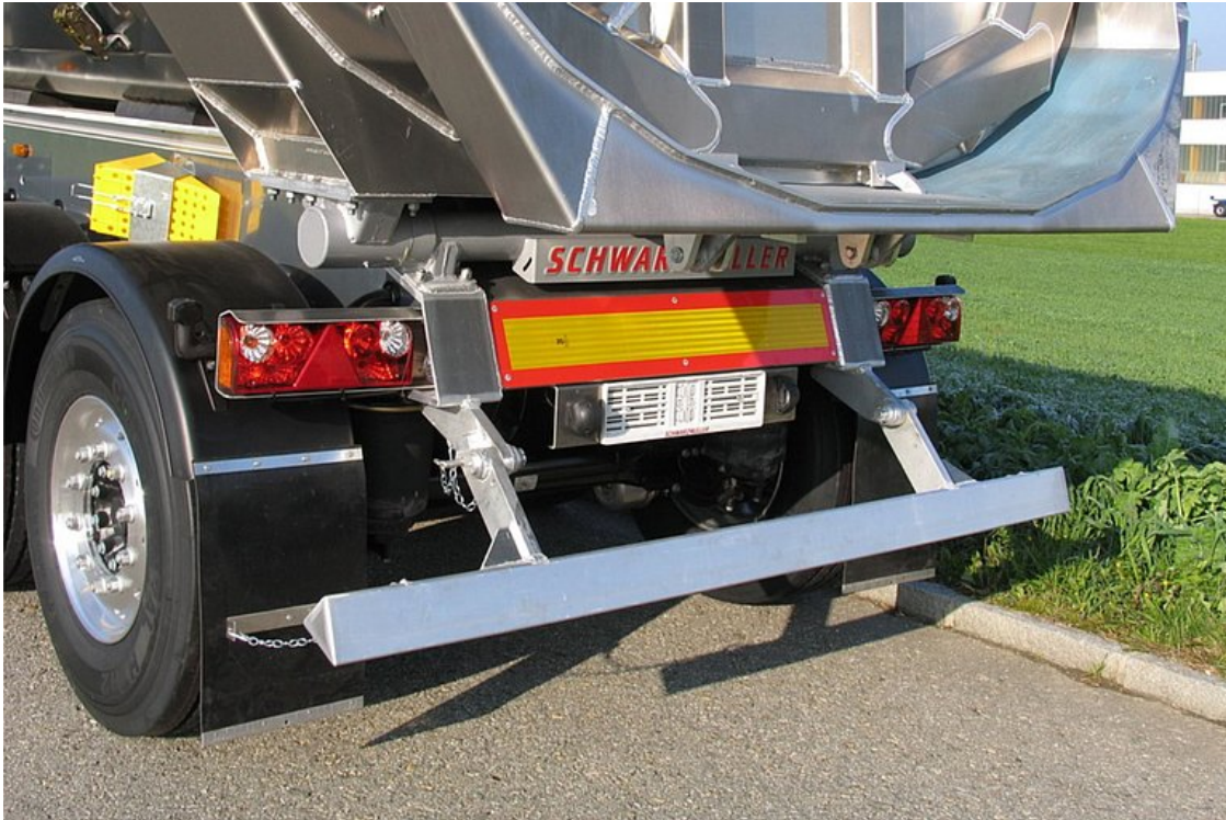
Foldable aluminium trapezoidal underride protection
