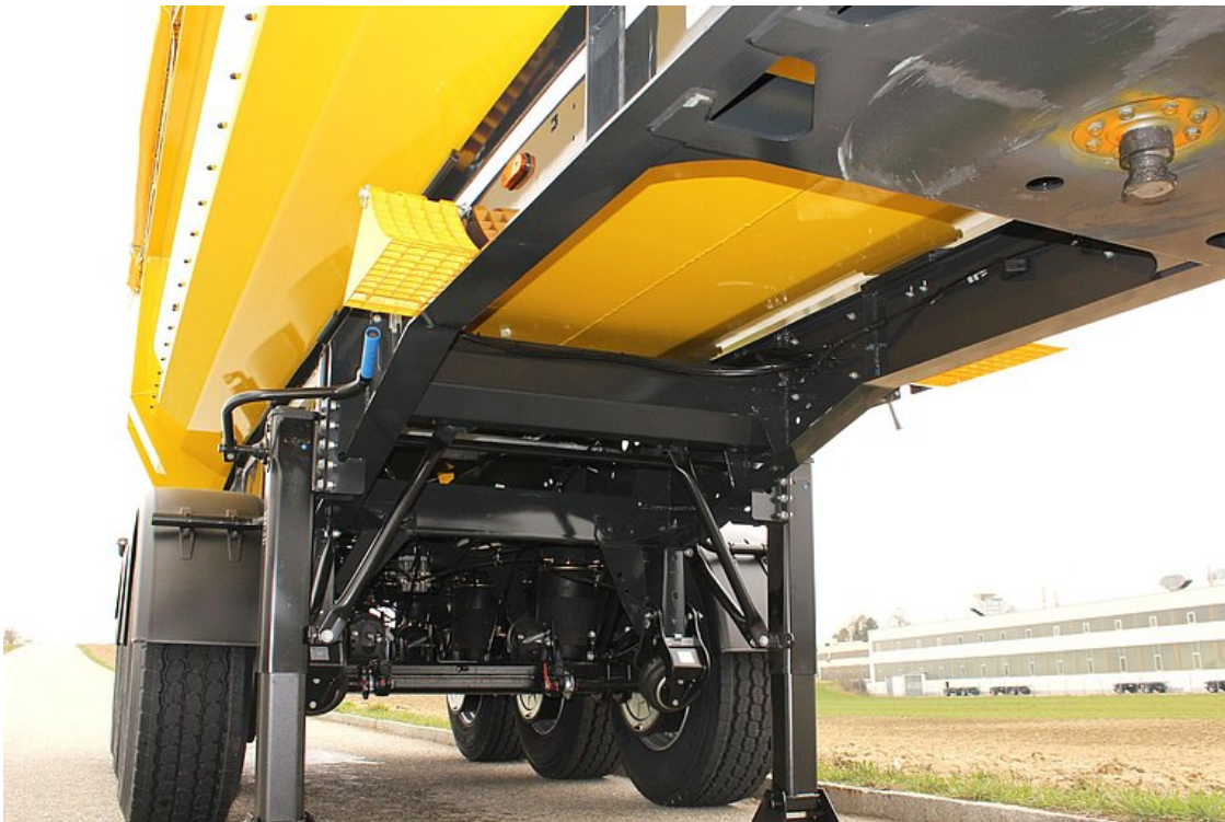
Stable and torsionally rigid chassis design with additional torsion tubes
