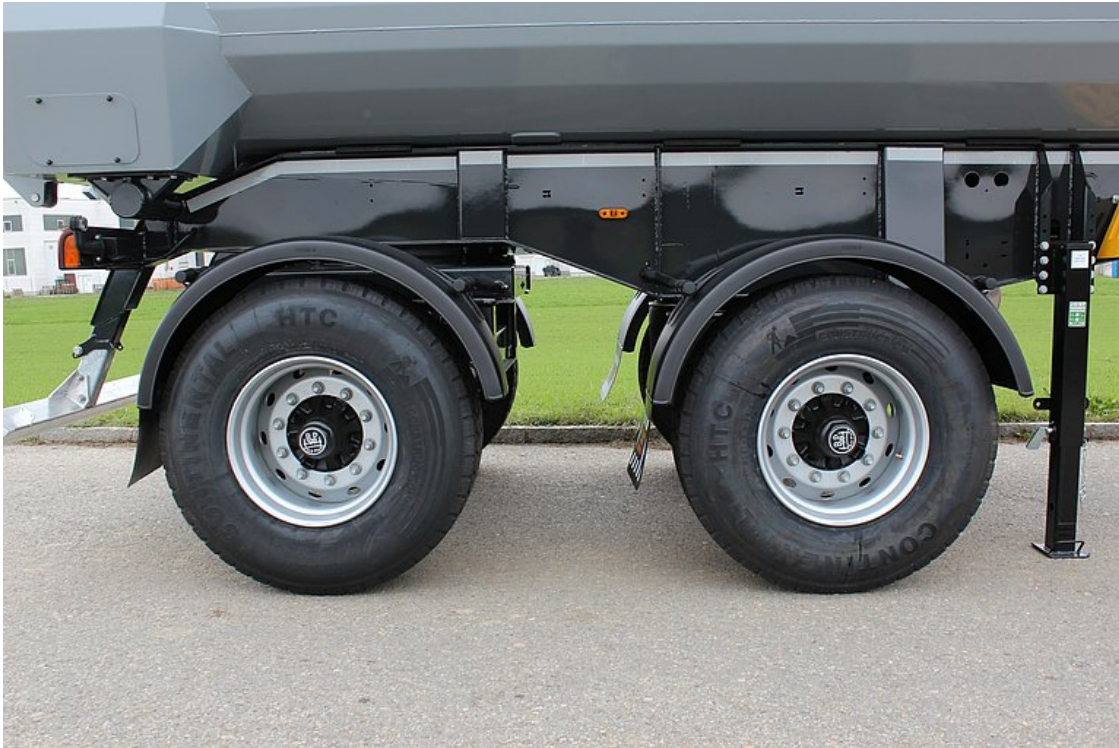
Axles with a wheelbase of 1,810 mm
