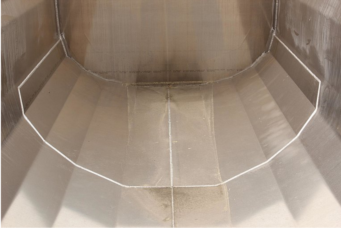
Aluminium wearing flooring in the rear area approximately 3,500 mm from the end of the bulk discharge chute
