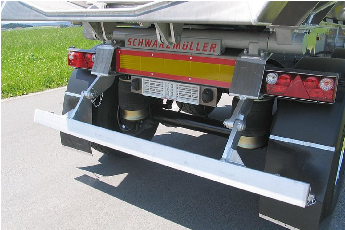
Foldable aluminium trapezoidal underride protection
