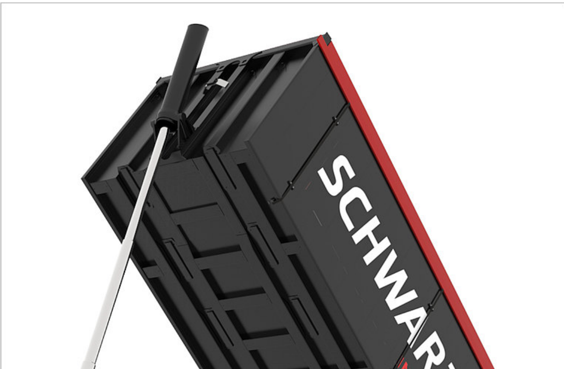
Four-point support: The press tipping mechanism is supported at four points (two at the top and two at the bottom). This substantially improves tipping stability compared to a three-point support.
