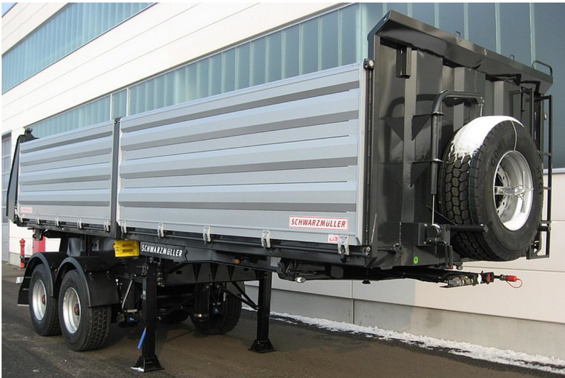
2-axle 3-way tipper semitrailer - building site
