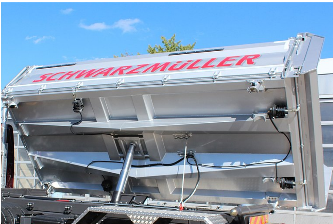
Conical trapezoidal profile side members in high-strength, lightweight design with small bottom panels for high dent resistance and shock absorption
