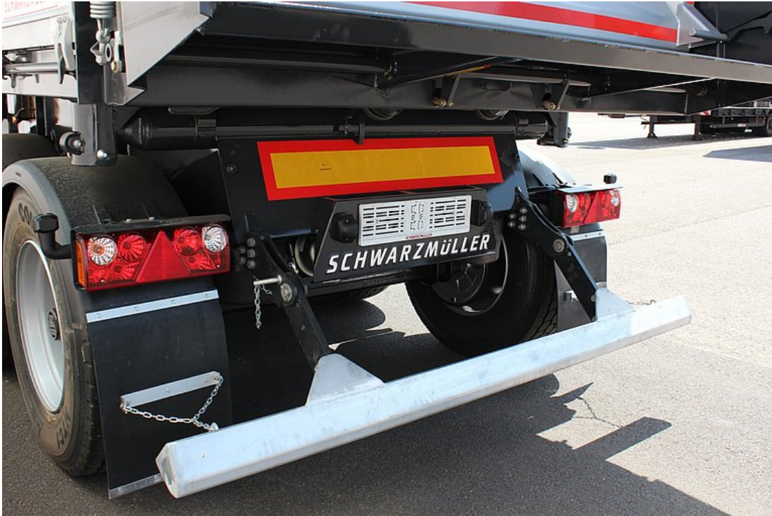
Foldable underride protection for road-finishing use
