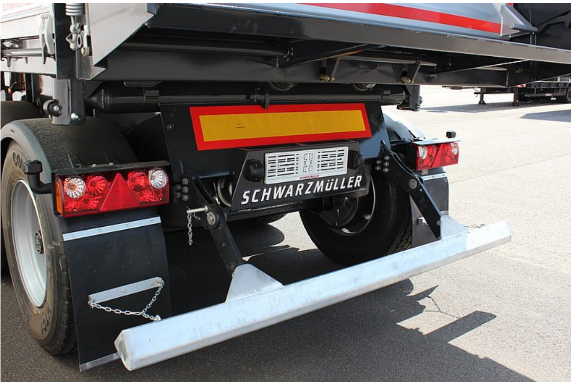
Foldable underride protection for road-finishing use
