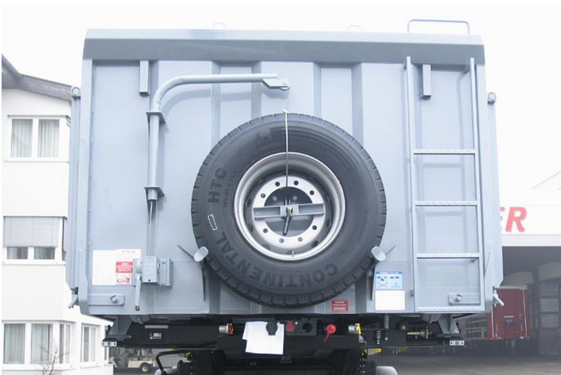
OPTIONAL: Spare wheel bracket with swivel boom and winch on front wall
