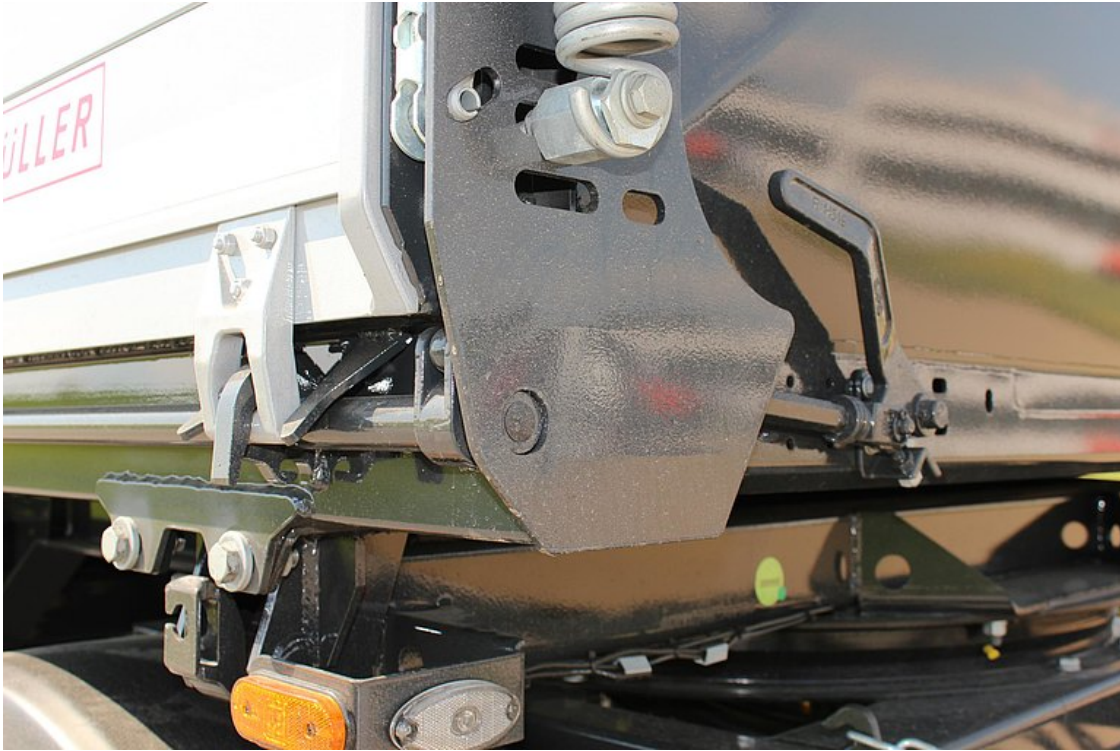
Manual central locking to open the side walls using a lever and central locking shaft
