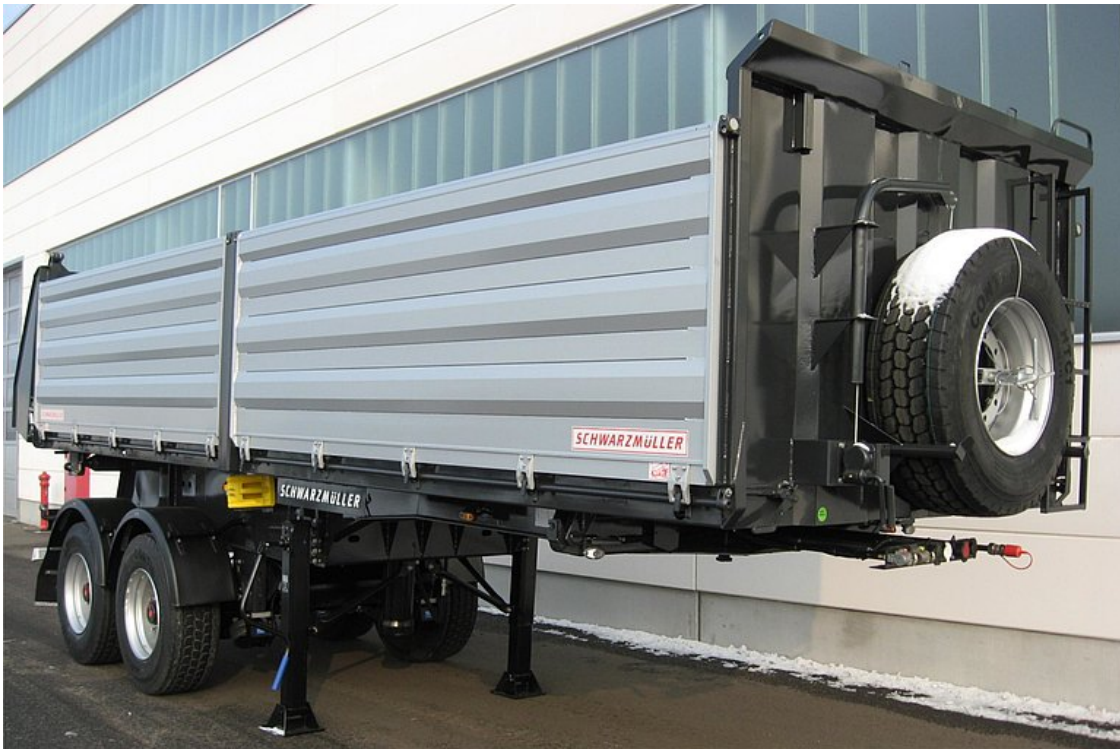
2-axle 3-way tipper semitrailer - building site - reinforced
