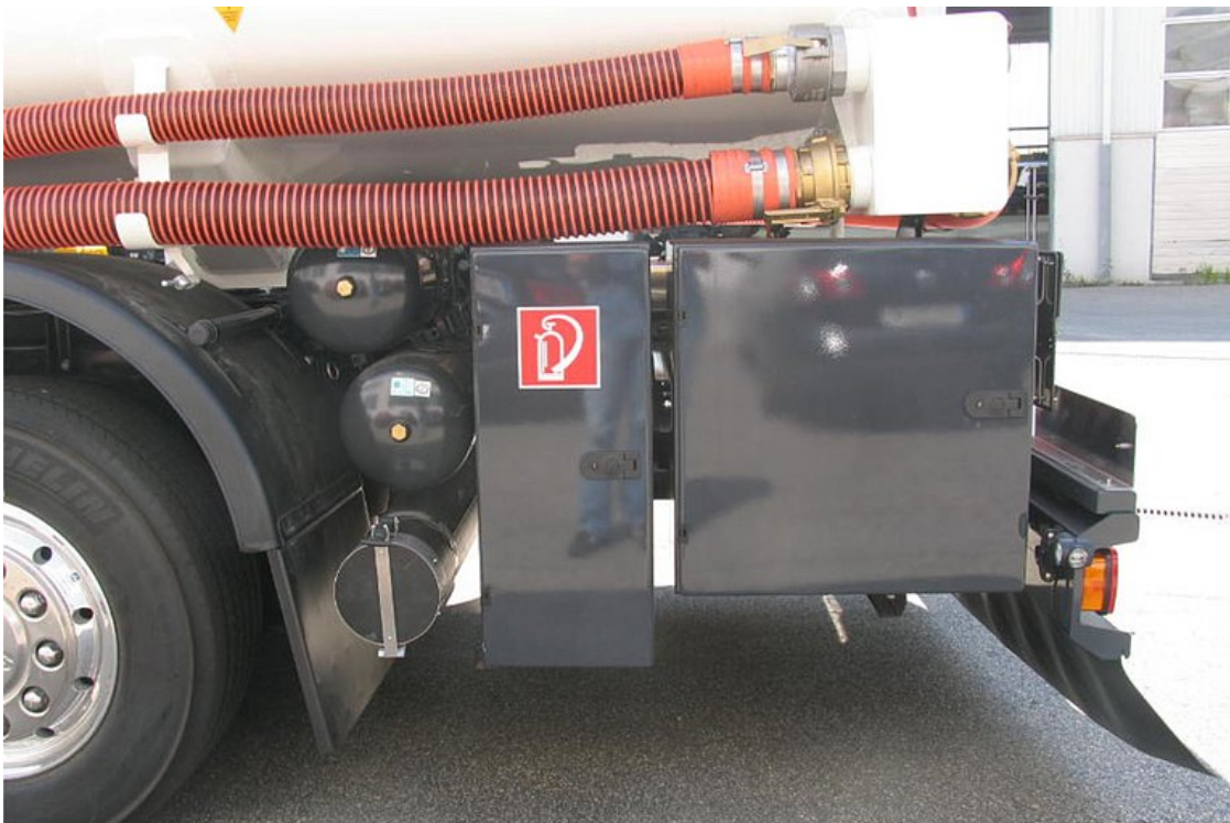
Aluminium box for 12 kg fire extinguisher and accessories box
