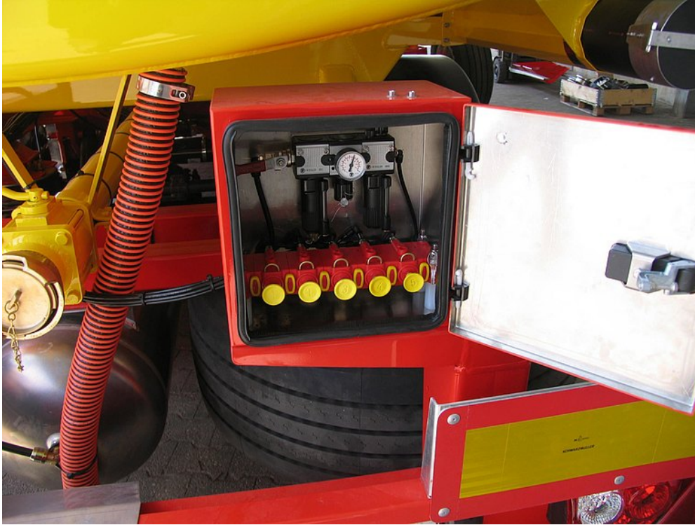
Box for pneumatic valve control to protect valves
