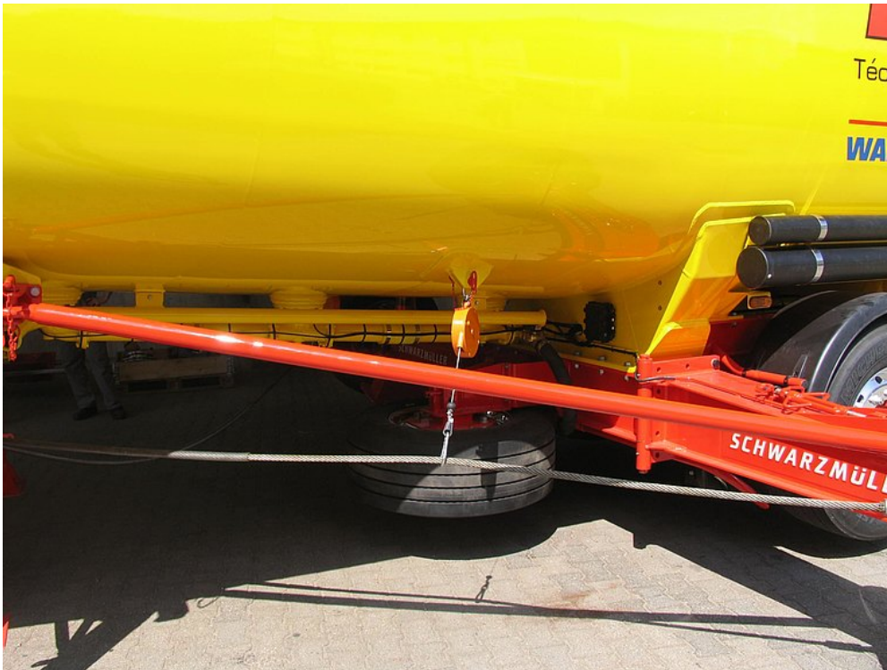
Anti-kink cables around the arm support towards the tank
