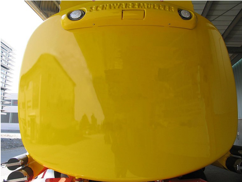
OPTIONAL: High-set LED light holder with optional integration of reversing camera
