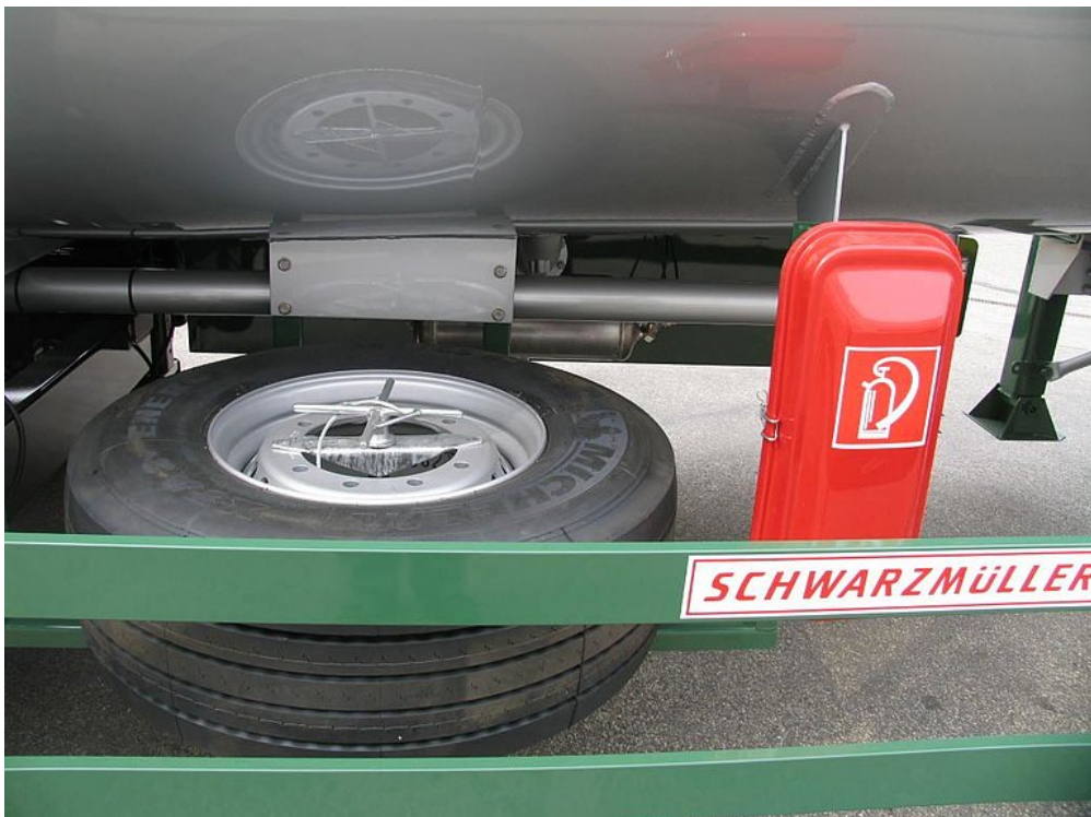
OPTIONAL: Facility for mounting spare wheel bracket
