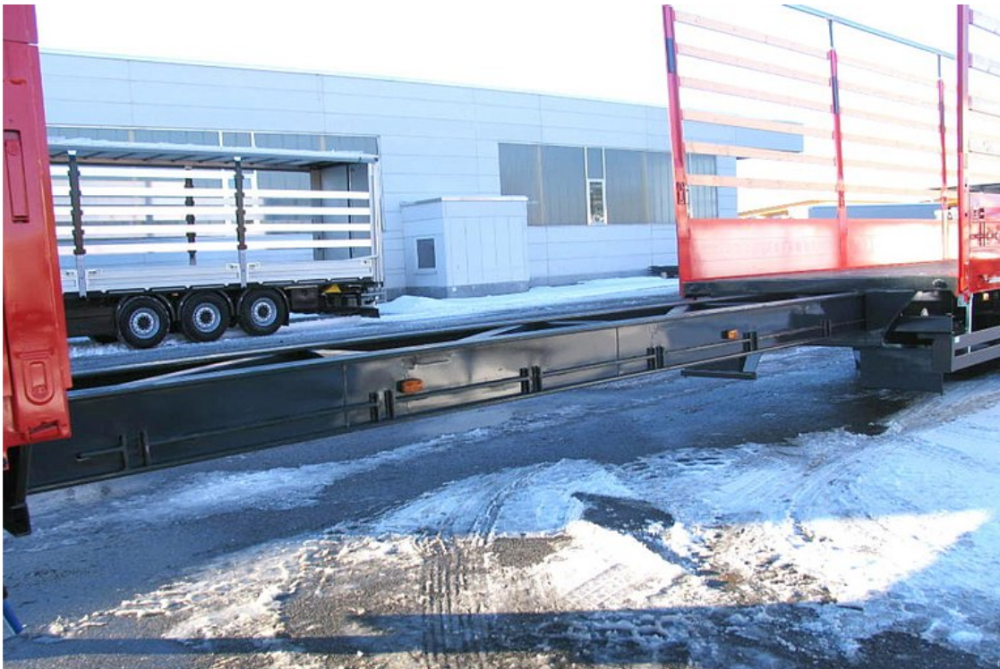
Torsionally rigid, pull-out welded steel frame design, with 7-step pneumatic locking
