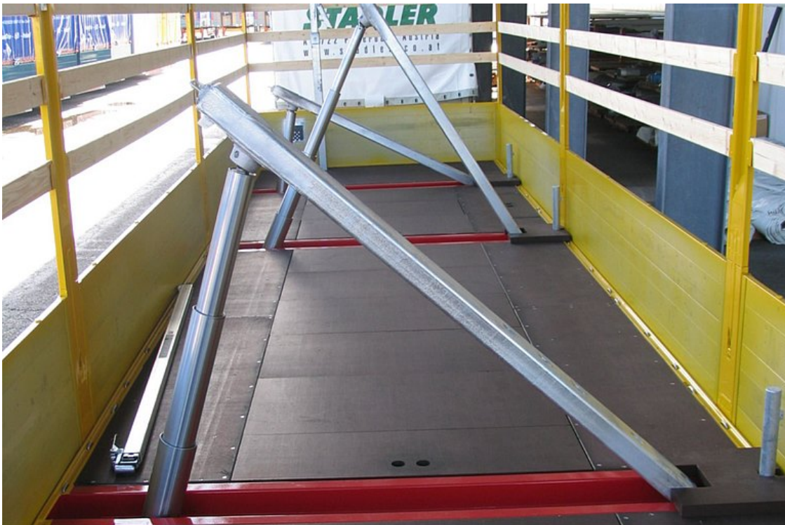
Hydraulic inclined loading device to transport large-format sheet metal up to 3,300 mm wide
