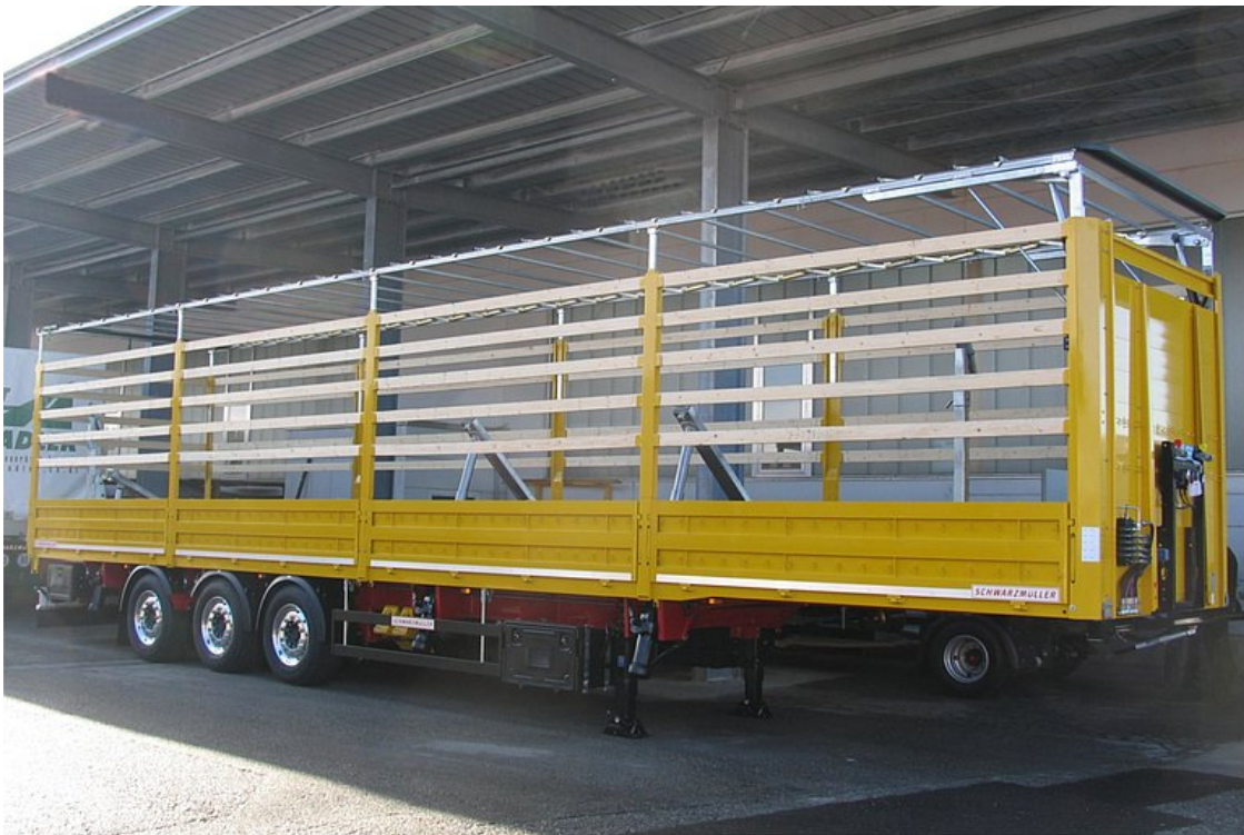
3-axle lightweight platform semitrailer - coil - inclined loader
