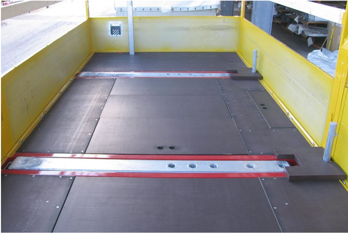
Load area with retracted inclined loading device
