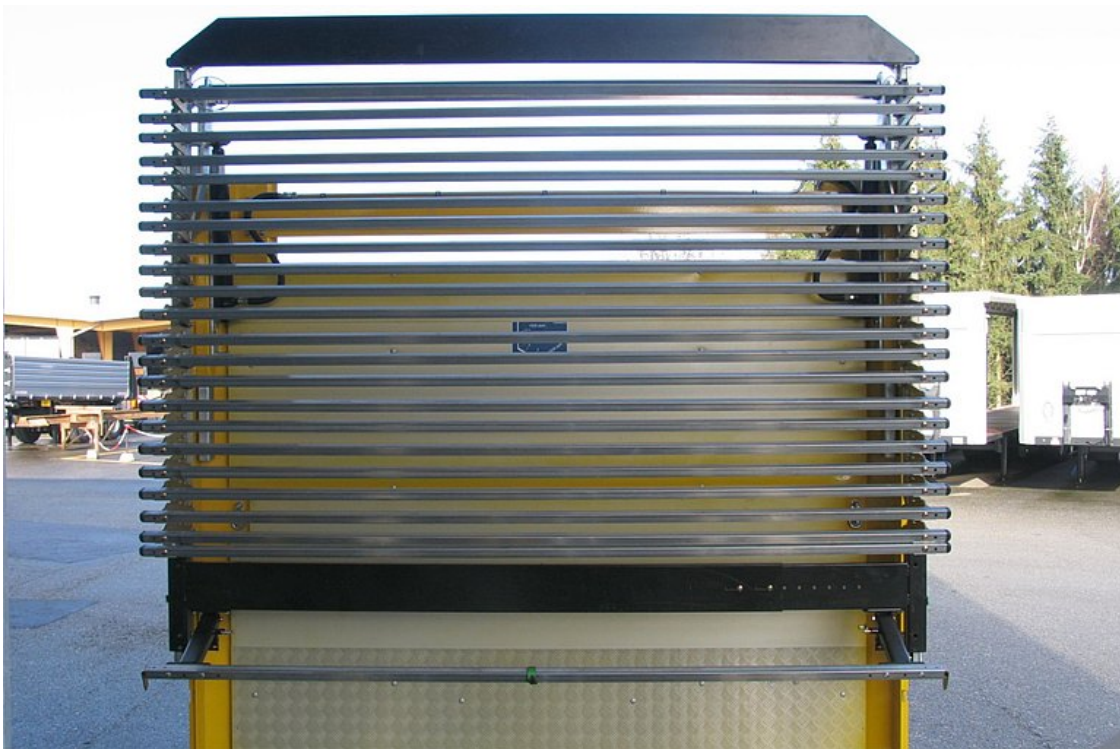
Sliding cover, hydraulically foldable against inside of front wall for open plate transports
