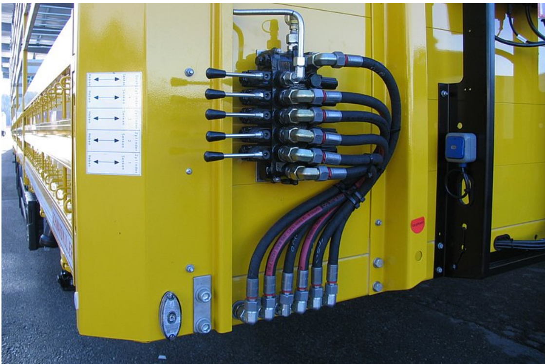
Hydraulic control unit for inclined loading system
