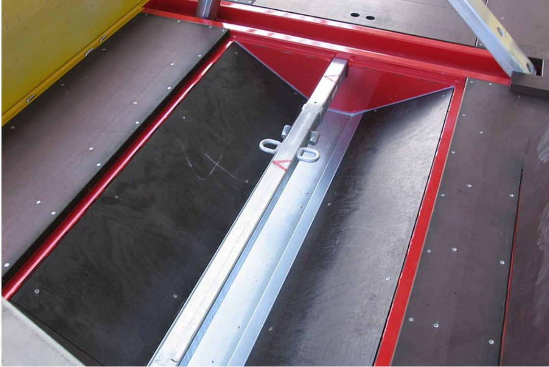
Coil recess with useful length of approx. 8,000 mm (split into 3 segments) - for coil diameters of between 900 and a max. of 2,100 mm
