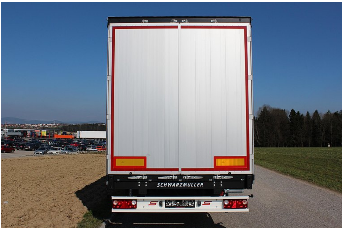
Bolted portal at rear with aluminium corner posts and fully opening double door in profile design
