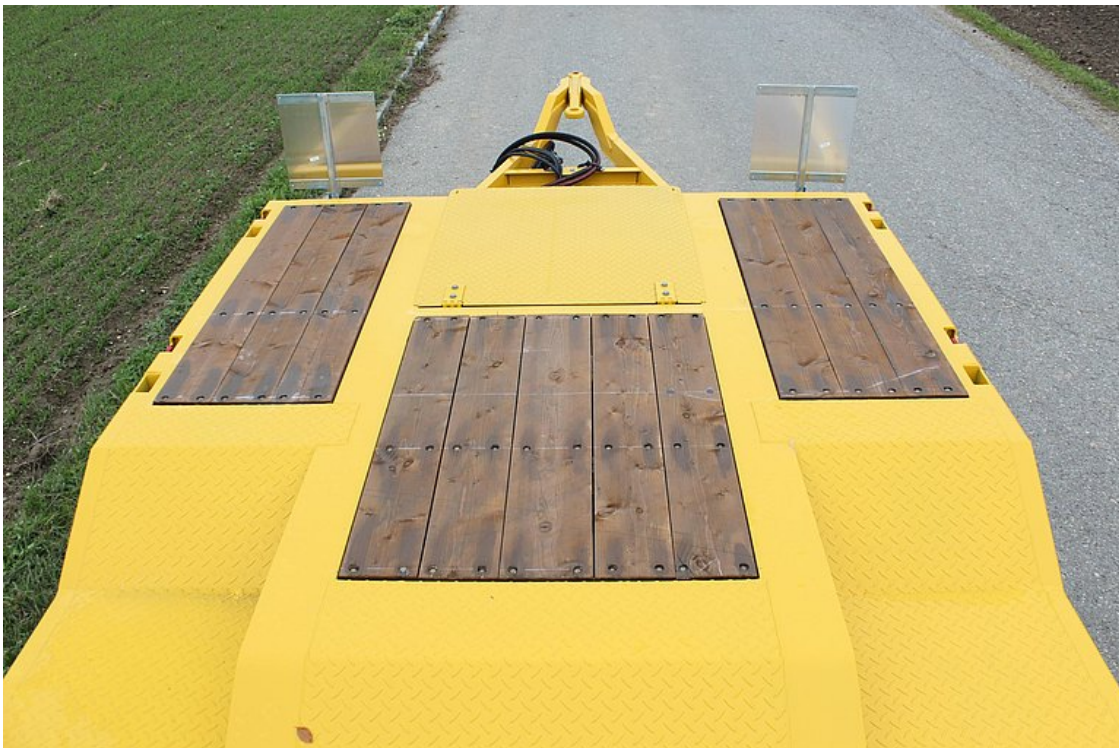
Raised platform at the front incl. offset frame, tapered corners
