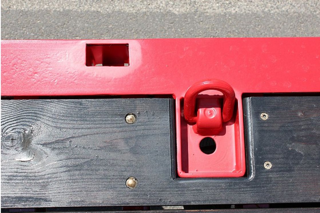
5 pairs of recessed, foldable lashing eyes
