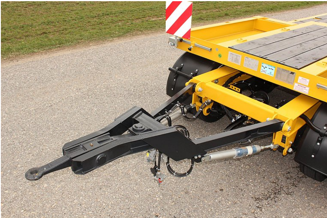
Offset drawbar with pivoting eye, 40 + 50 mm
