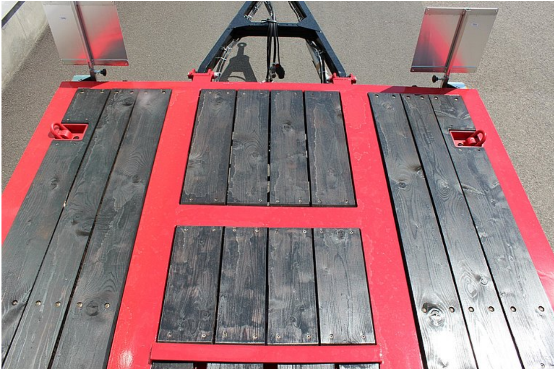
Waterproofed softwood floor, protruding beyond frame profiles
