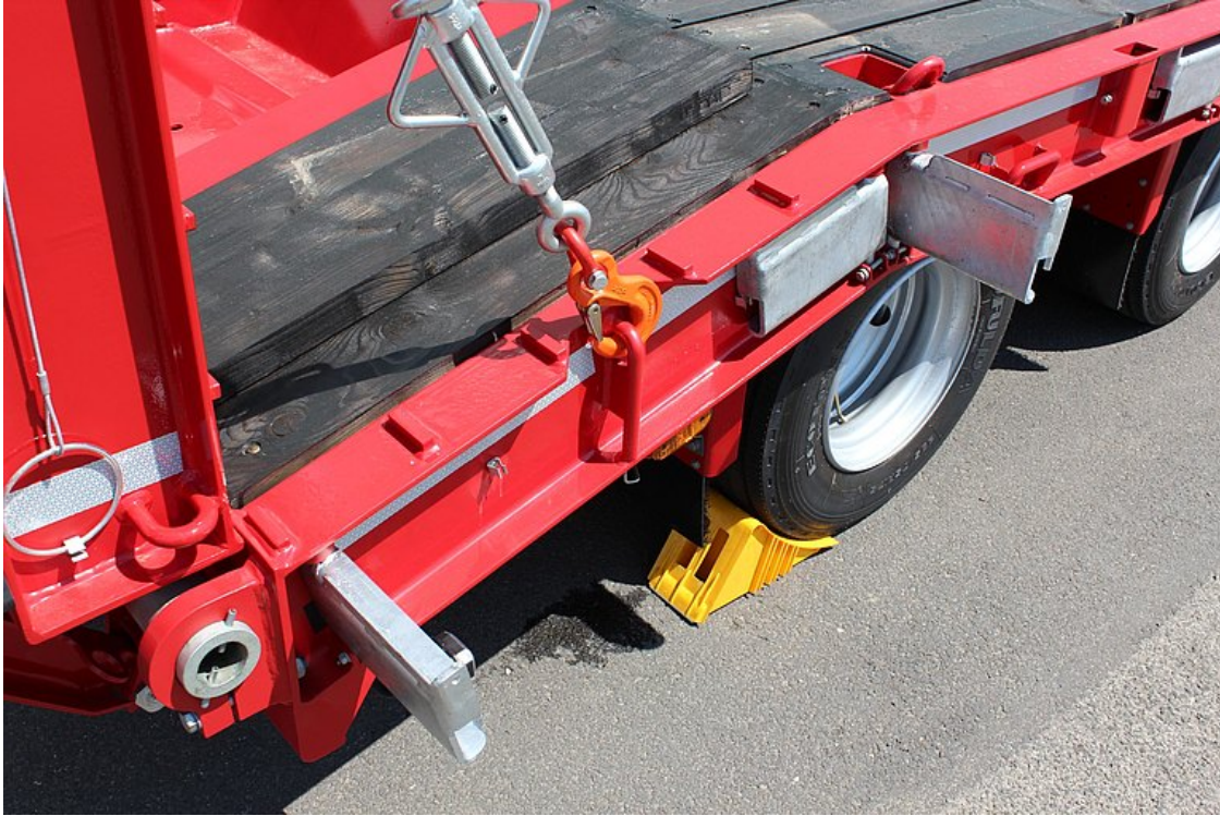
OPTIONAL: Foldable, pivoting extensions, incl. extension planks for transporting wide loads
