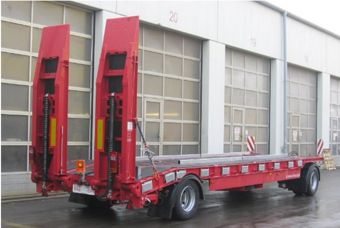
2-axle low loader trailer with straight platform
