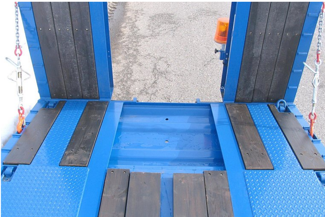
OPTIONAL: Excavator shovel recess between side members at rear
