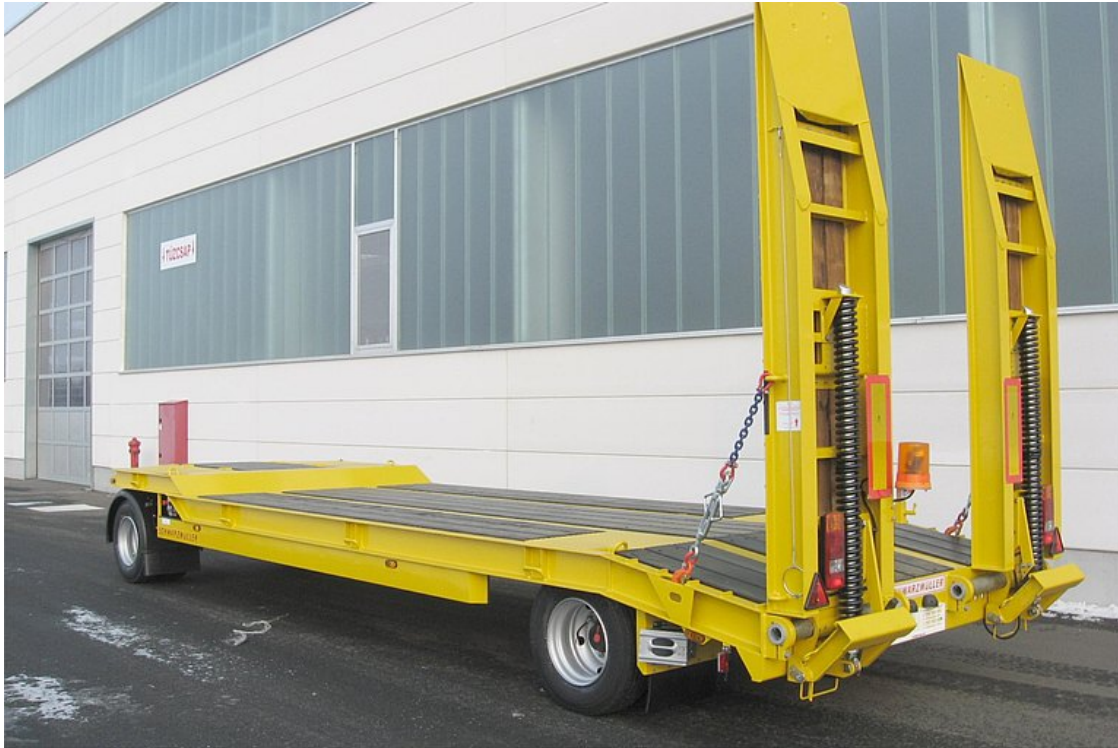
2-axle low loader trailer with offset platform
