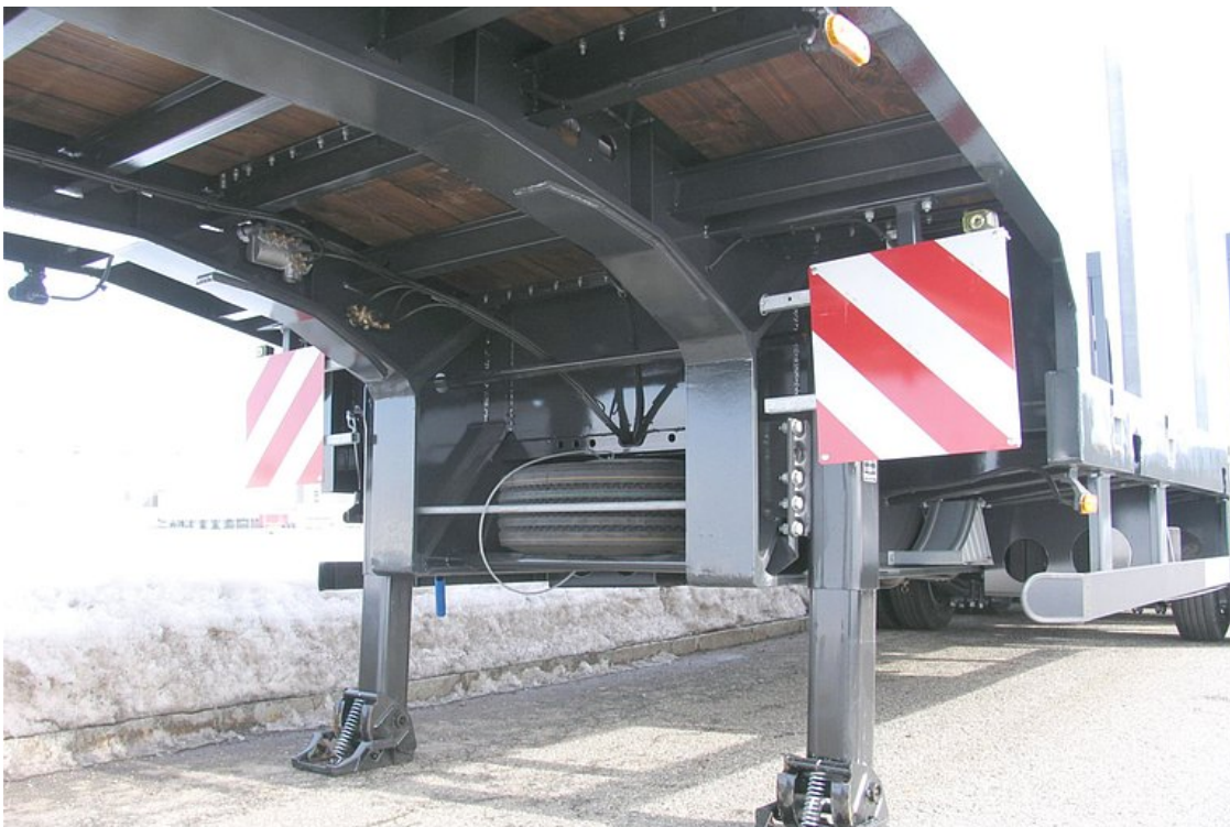
Reinforced and torsionally rigid welded steel design with narrow cross member spacing for high point loading
