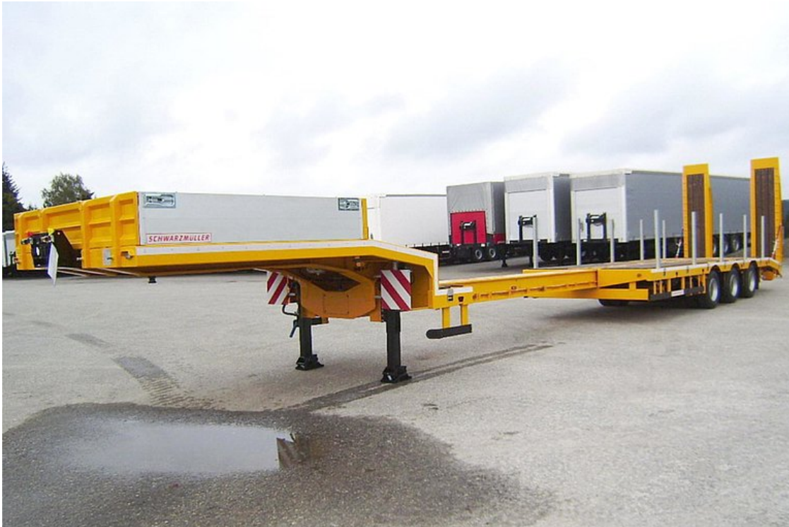
3-axle low loader semitrailer - reinforced - extendible
