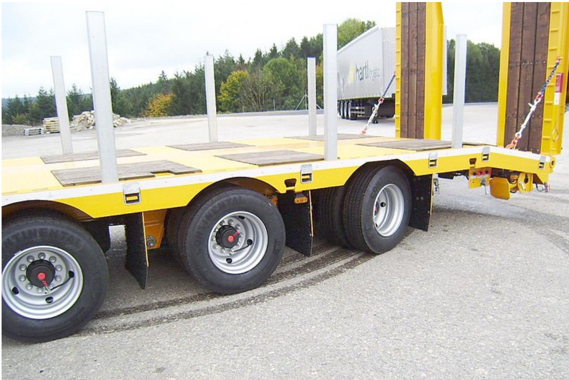
Third axle is steered trailing axle for improved cornering and lower tyre wear
