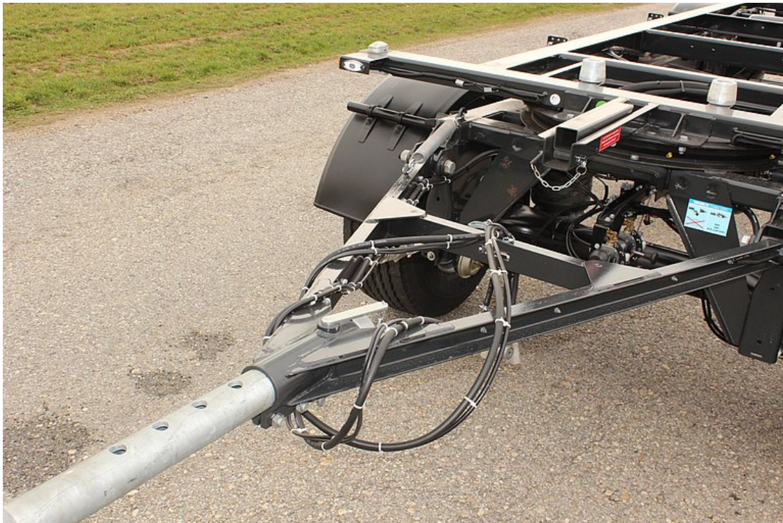
Pull-out drawbar, max. 600 mm adjustment, with Getofix drawbar support
