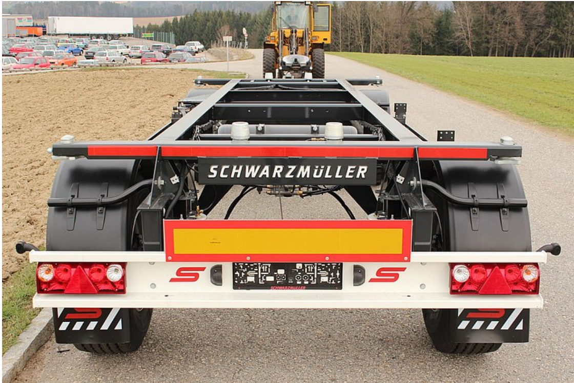
Underride protection incl. integrated light system
