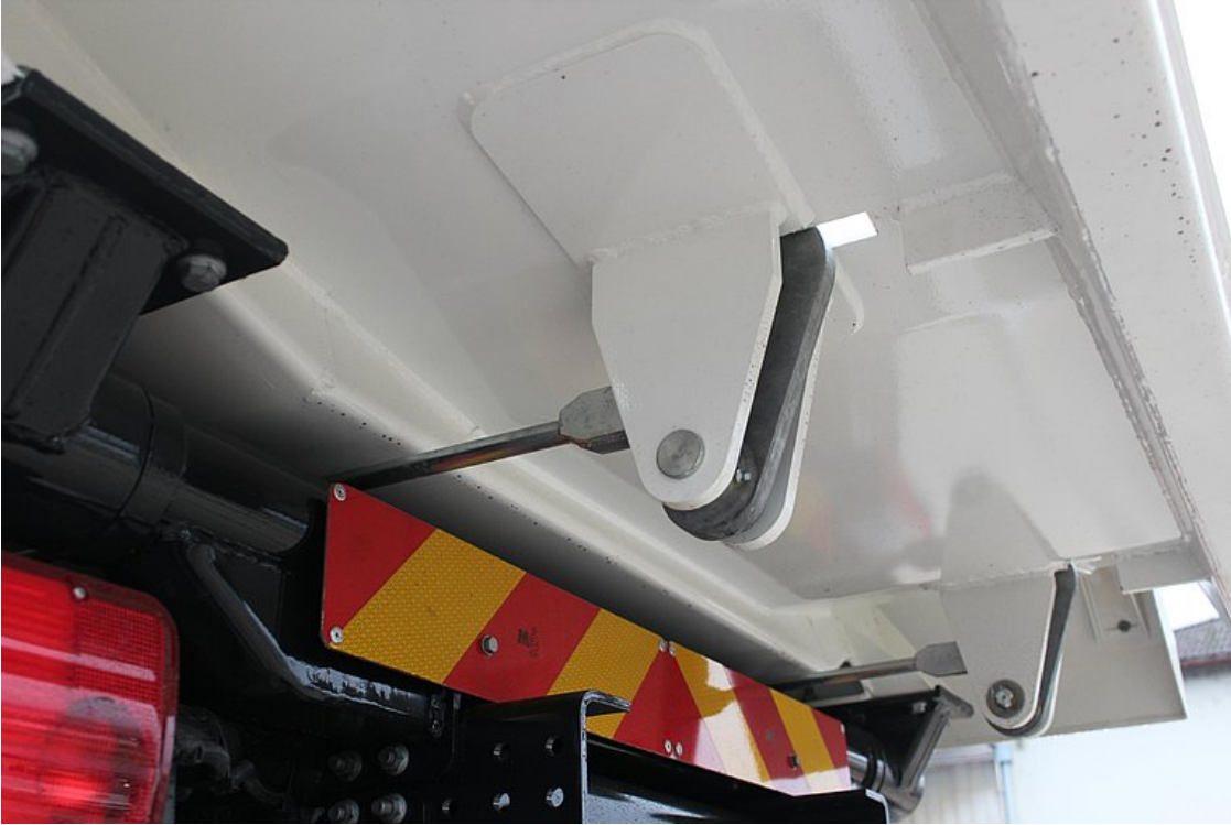
Automatic mechanical rear wall locking
