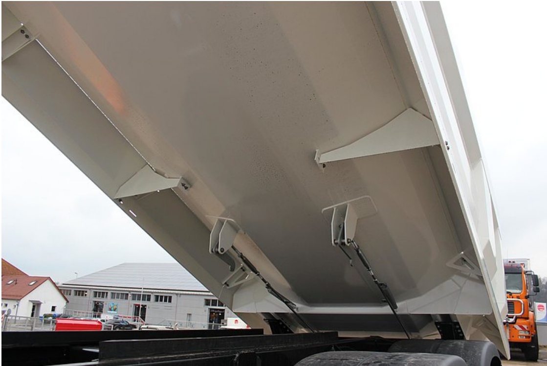
Specially canted Hardox body for maximum impact and wear protection
