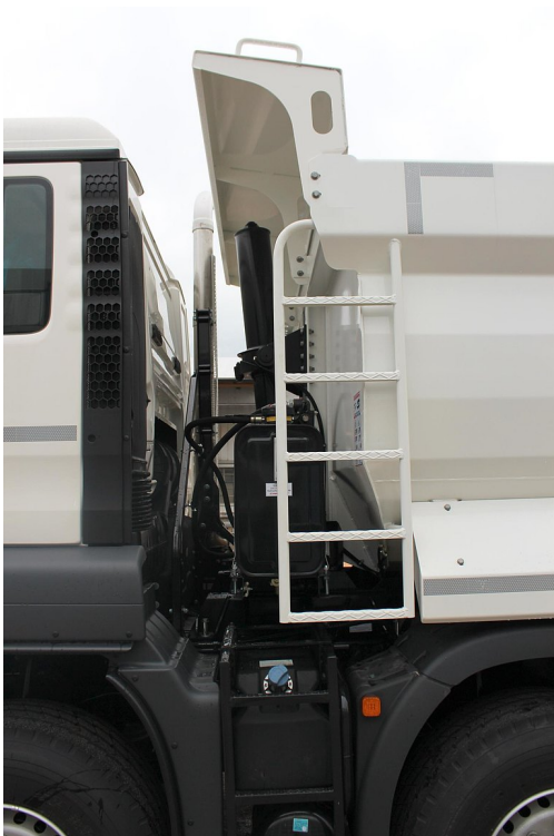
Fixed ladder on outside front left side
