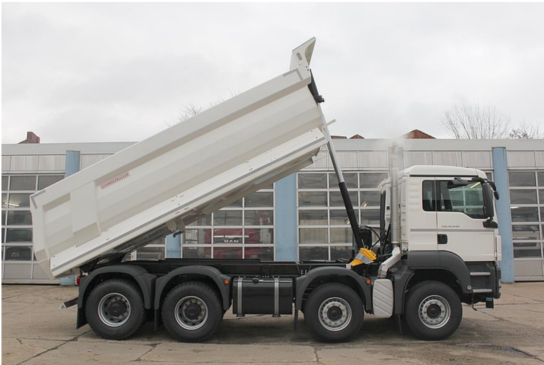
Steel segment tipper body on 4-axle truck
