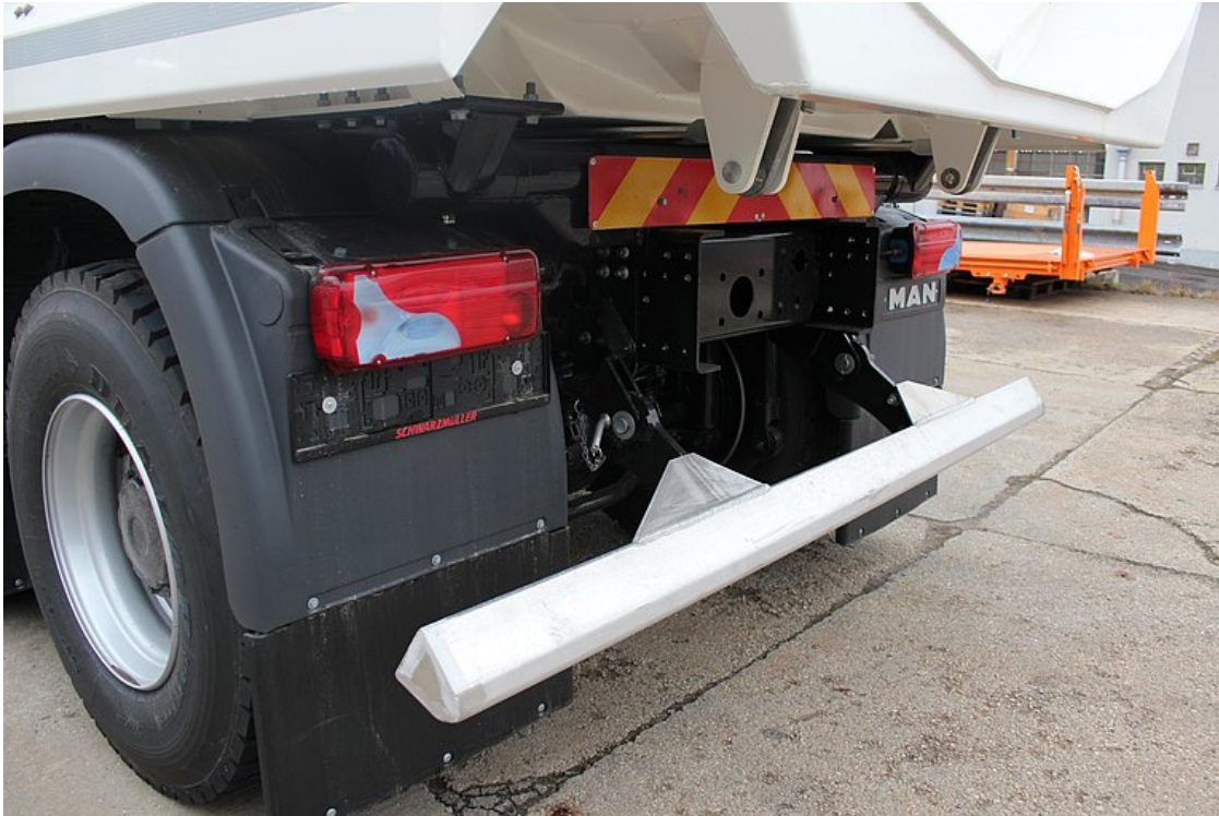
OPTIONAL: Foldable aluminium underride protection
