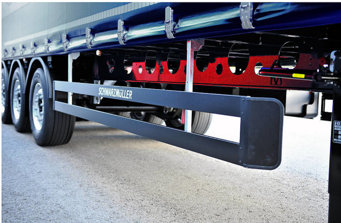
Side impact protection: Statutory cyclist protection to prevent persons from falling down in front of the wheels.
